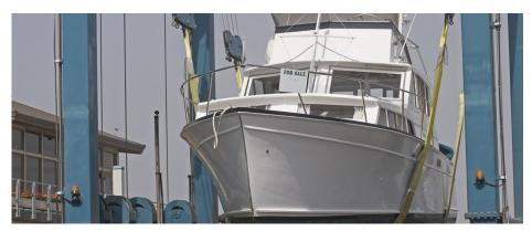
Boat hoist slings are an often overlooked yet critical component of your boat hoist system. These synthetic web slings, made of either nylon or polyester, are susceptible to many deteriorating or damaging conditions during regular use. Effective protocols for sling inspection, care, and replacement must be in place to prevent potential damage, injury, or death from sling failure.
